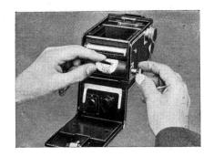
3. Detach the gummed strip of the film spool and lead the paper over the guide roller (v) and insert the tapered end into the slot provided in the empty spool on the other side of the camera.
