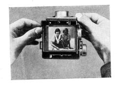
3. If it is required to hold the camera in a rather high position, the exposure may be made at eye-level.
