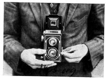
For the longer instantaneous exposures it is useful to steady the camera with the left hand as shown.
